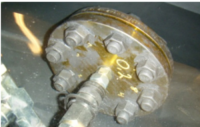
Figure 6 – Assembled test sample for gaseous helium testing (One flange with groove and one smooth flange)
