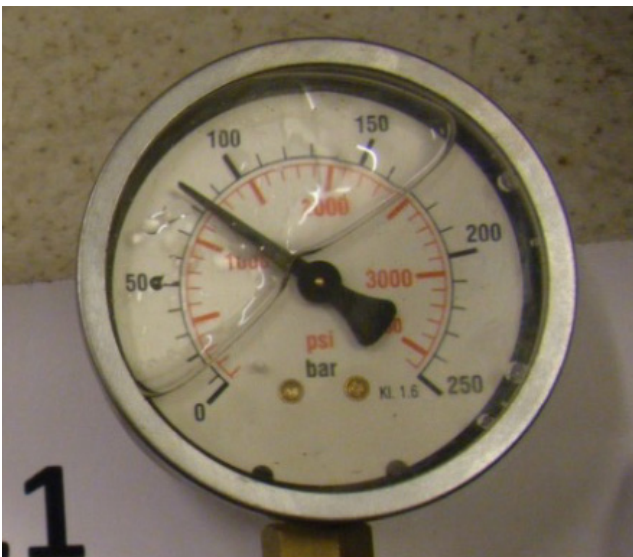
Figure 10. Water testing - 78 barg
