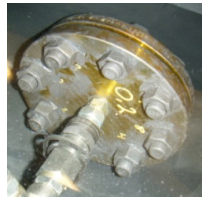
Figure 14. Helium testing - 5 barg
