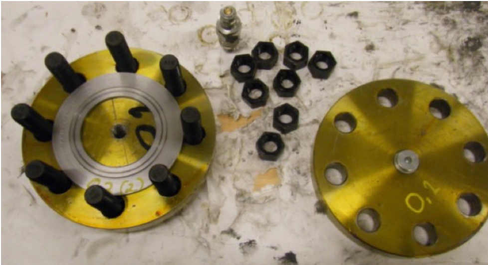
Figure 11. Assembly of test specimen
