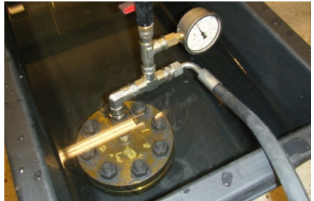
Figure 18. Helium testing - 5 barg - No detected leakage at 108 Nm torque
