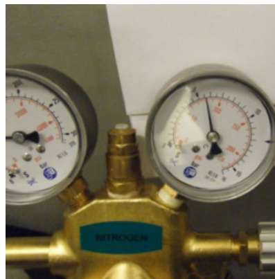
Figure 13. Helium testing - 5 barg
