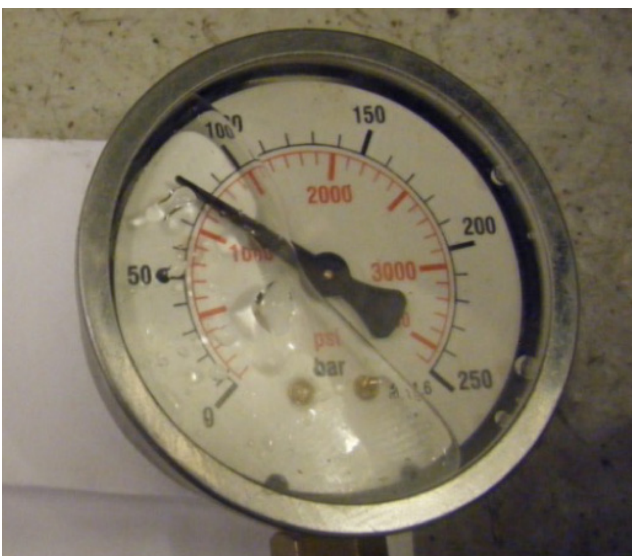
Figure 15. Water testing - 78 barg
