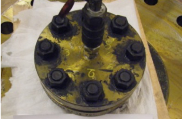
Figure 8. Helium test - 5 barg
