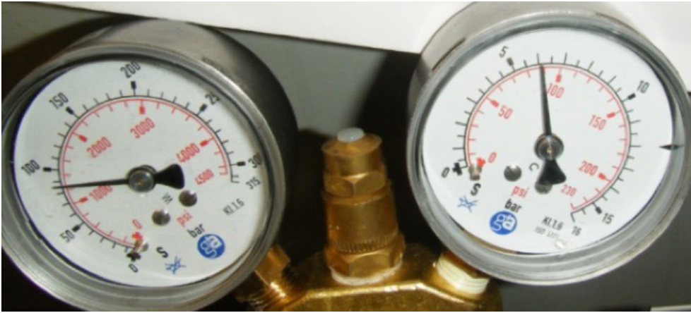
Figure 16. Helium testing - 5 barg
