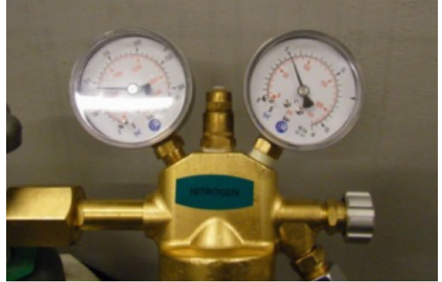
Figure 9. Helium test - 5 barg
