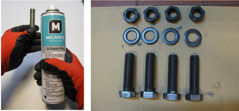
Fig. 8 Lubrications of the fasteners
