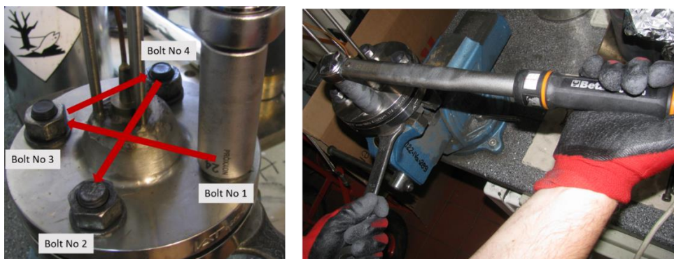
Fig. 10 Bolt tightening sequence
