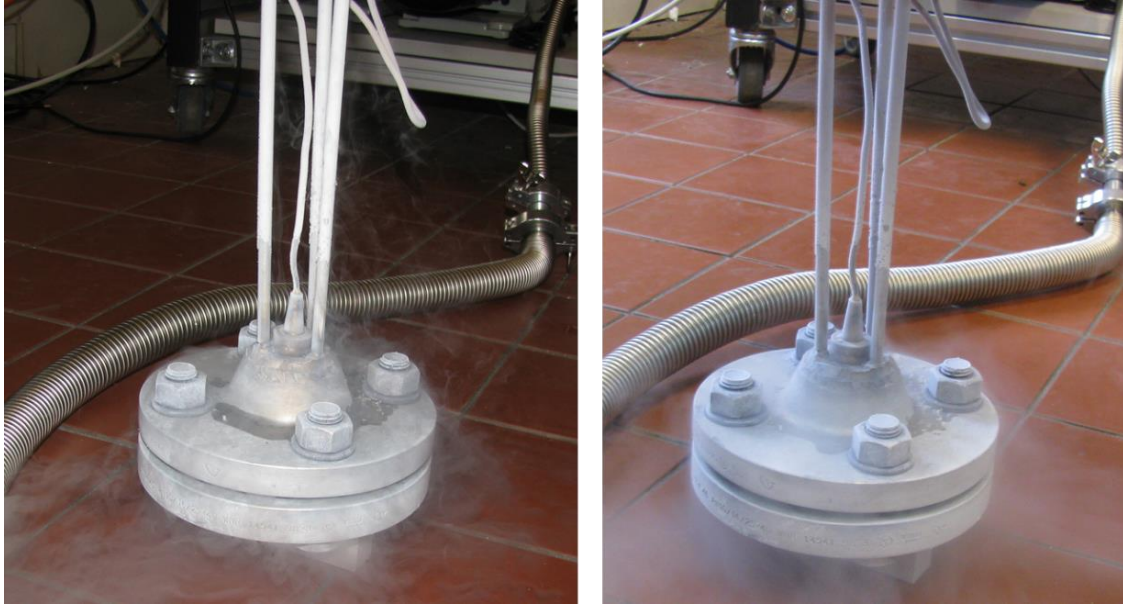
Fig. 11 Flange joint after immersing in liquid nitrogen
